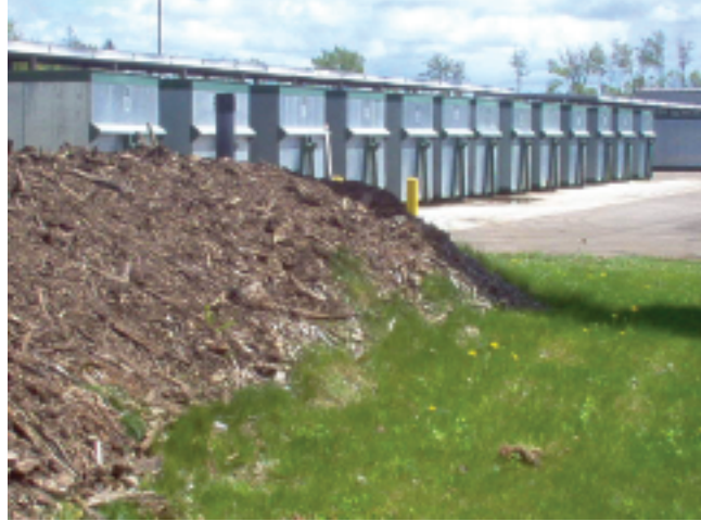
The site has 52 composting vessels. Compost stays in the vessels for 10-14 days.
