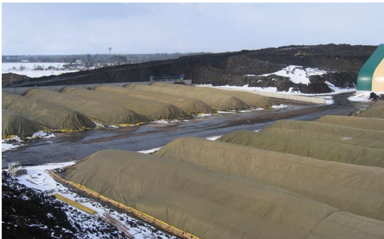
The GORE material helps insulate the piles from rain and snow, but the material breathes enough to help prevent the material from going anaerobic.
